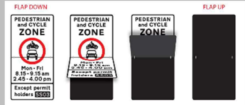
Two regulatory signs are installed at each entry point. Outside of term, signs are closed and School Street does not operate
